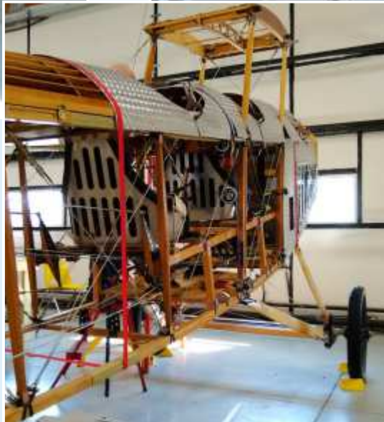
Seats mounted and control wires installed.
