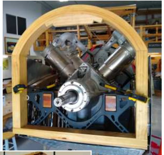
The hundred-year-old liquid-cooled V-8 power plant produces just 90 hp. It is shown above temporarily installed..
