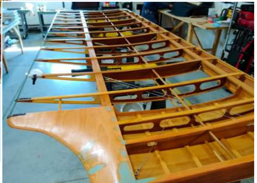
A constructed wing being prepared for covering
